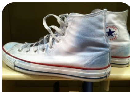
Dye from dyed textile rubs off on adjacent substrates
