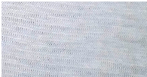
Fabric soaked in beaker containing Chelatin-SA shows very less Iron stains as compared to Blank
