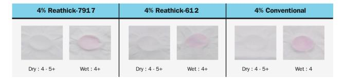
Reathick-7917 and Reathick-612 shows comparable printing effects against Conventional printing with sodium alginate thickener.
