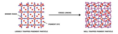
After evaporation of the solvent or other liquid vehicle, heating produces a thin coating or film. The film, several microns in thickness, encloses the pigment particles and adheres to the fibre. Since pigment coloration is an additive effect to the
