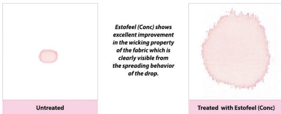
Absorbency efficiency of Estofeel(Conc) finished fabric by drop test
