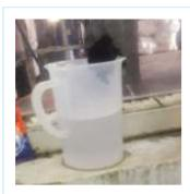
The reactive dyed yarn is soaped with Sarakol-0472. The soaped yarn was dipped in water and checked for any bleeding taking place. As clearly seen from the photograph, the water is absolutely clean which justifies the washing off efficiency of Sarakol-0472.
