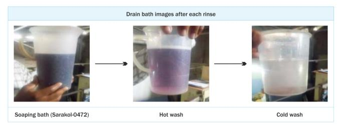
The final cold wash rinse is clean and clear which proves the efficiency of Sarakol-0472
