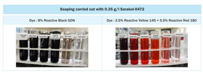
The final cold wash rinse is clean and clear which proves the efficiency of Sarakol-0472
