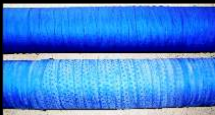
Fig. Beam dyeing of Blue shade on polyester with and without Eliminator GLO
